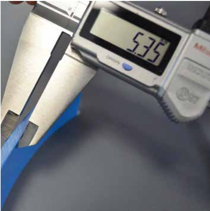
Accurate measurement of a test specimen using a calibrated caliper
