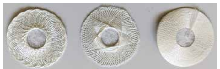
Fig. 3: Textile reinforcing structures produced by the TFP process
